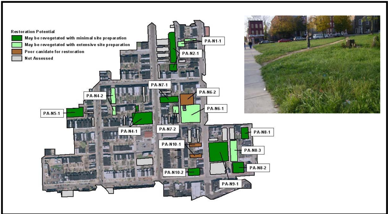
Figure 5.3: Restoration potential of pervious areas identified during the USSR in a subwatershed of Watershed 263 in Baltimore, Maryland
