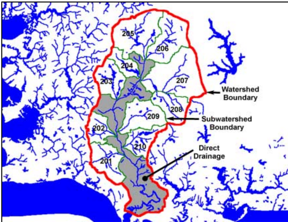
Figure 6: Subwatershed and Direct Drainage (shaded) Delineation for the Powhatan Creek Watershed in James City County, Virginia
