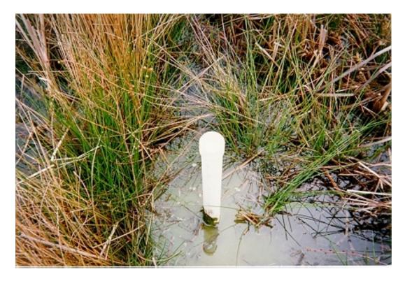
Figure 3.1: Groundwater monitoring well used before construction and also through monitoring after construction (photo Noble)
