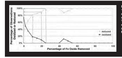
Fig. 6. The proportion of Fe oxide paint removed from a 10-cm (4-inch) section of IRIS tube related to the percentage of Eh pH observations where the soil was reduced or oxidized according the Technical Standard of the National Technical Committee on Hydric Soils. Note that when 20% of the Fe oxide paint is removed from a 10-cm (4-inch) zone, the soil was reduced in 90% of the observations. Modified from Castenson and Rabenhorst (2006).
