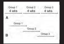
Fig. 4. (A) Groups of IRIS tubes are installed for approximately 4 wk, after which a replacement set can be reinstalled. (B) For better temporal resolution, groups of tubes can be installed at 2-wk intervals so that the periods of installation overlap.
