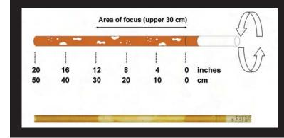
Fig. 5. Estimates of the proportion of the tube area where paint has been removed should be made while rotating the tube. When focusing on issues of hydric soils, the area of interest is the upper 30 cm (12 inches) of the soil.
