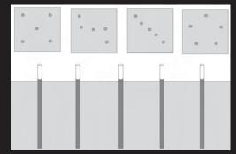
Fig. 3. Five replicate IRIS tubes should be inserted into a uniform area or "plot" that typically covers 1- to 2-m<sup>2</sup>. The tubes can be placed in any convenient arrangement that ensures their even distribution over the area of interest.
