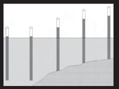
Fig. 2. IRIS tubes are typically inserted 50 cm (20 inches) into the soil unless rock, gravel, or some other impediment interferes. If the tubes cannot be inserted to 50 cm (20 inches), then a line should be drawn on the tube to indicate the location of the soil surface.
