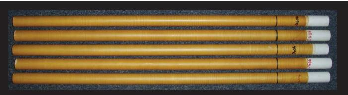
Fig. 1. Set of five IRIS tubes with line marking 50 cm (20 inches) from the bottom of the tube. The notation on the tube identifies the particular batch of paint used in making these tubes (0606).
