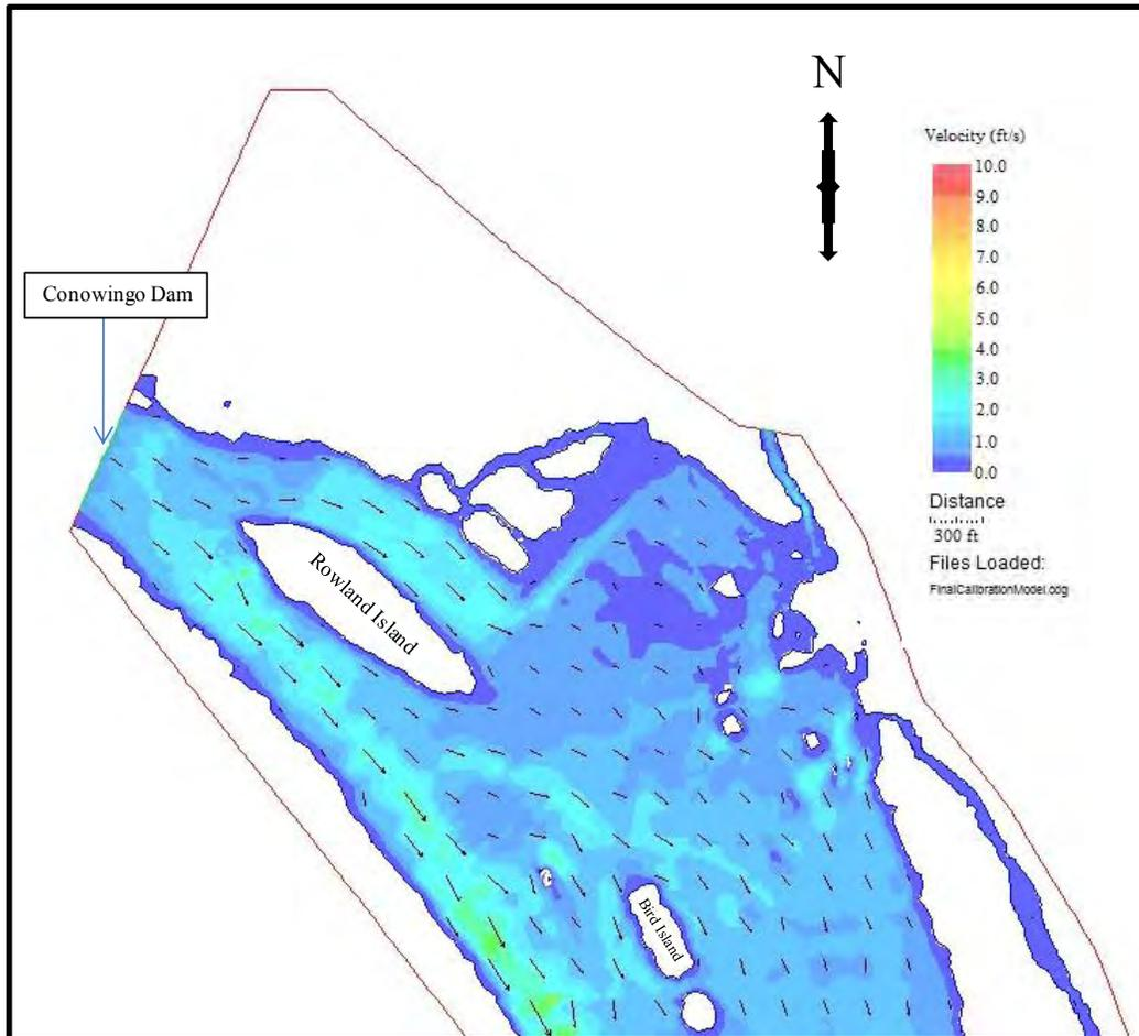
**FIGURE 4.2-3: WATER VELOCITY IN THE SUSQUEHANNA RIVER IN THE VICINITY OF BIRD ISLAND AND REUBEN ISLAND AS DETERMINED BY RIVER 2D MODEL FOR 10,000 CFS DISCHARGE FROM CONOWINGO DAM.**
