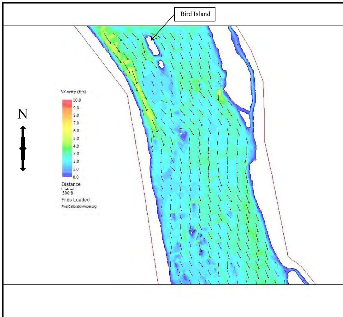
**FIGURE 4.2-9: WATER VELOCITY IN THE SUSQUEHANNA RIVER IN THE VICINITY OF REUBEN ISLAND AND ROBERT ISLAND AS DETERMINED BY RIVER 2D MODEL FOR 40,000 CFS DISCHARGE FROM CONOWINGO DAM.**
