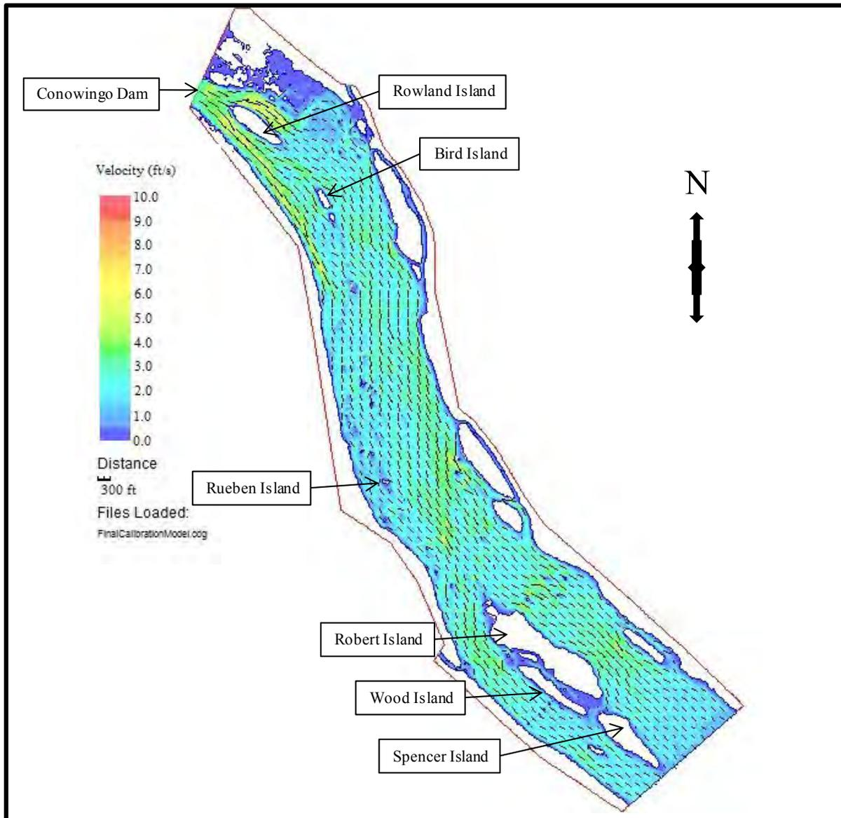
**FIGURE 4.2-7: WATER VELOCITY IN THE SUSQUEHANNA RIVER IN THE VICINITY OF ROWLAND ISLAND AND BIRD ISLAND AS DETERMINED BY RIVER 2D MODEL FOR 40,000 CFS DISCHARGE FROM CONOWINGO DAM.**
