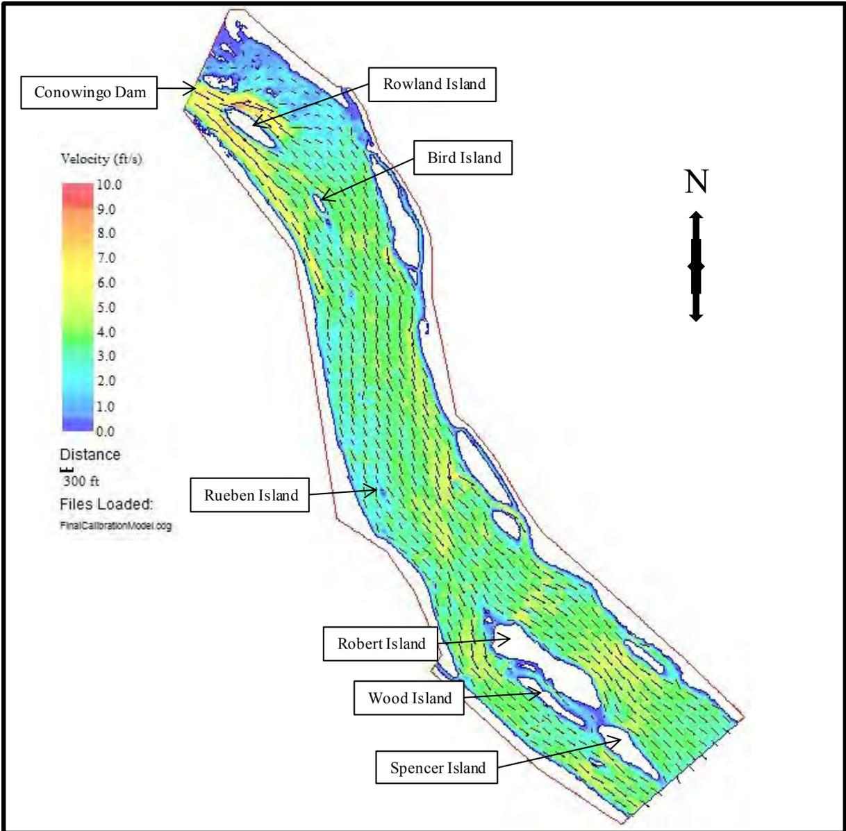
**FIGURE 4.2-12: WATER VELOCITY IN THE SUSQUEHANNA RIVER IN THE VICINITY OF ROWLAND ISLAND AND BIRD ISLAND AS DETERMINED BY RIVER 2D MODEL FOR 86,000 CFS DISCHARGE FROM CONOWINGO DAM.**
