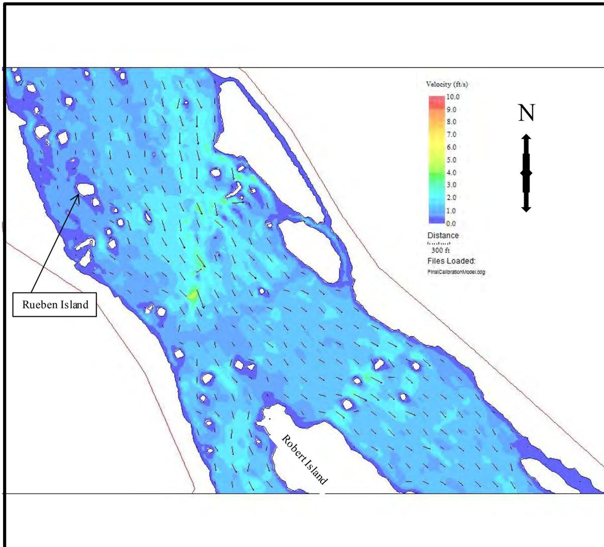
**FIGURE 4.2-5 WATER VELOCITY IN THE SUSQUEHANNA RIVER IN THE VICINITY OF SPENCER ISLAND AND ROBERT ISLAND AS DETERMINED BY RIVER 2D MODEL FOR 10,000 CFS DISCHARGE FROM CONOWINGO DAM.**
