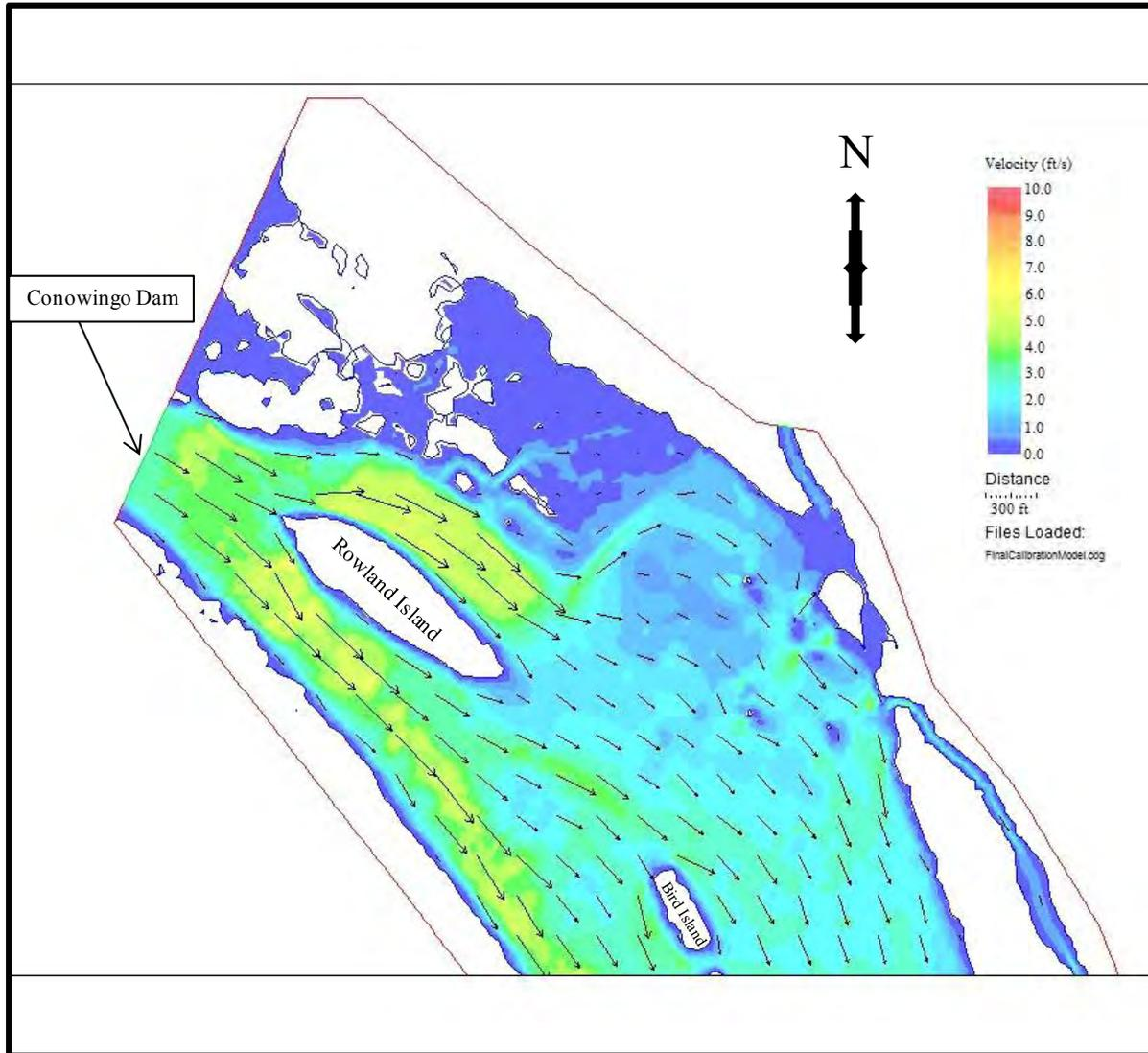
**FIGURE 4.2-8: WATER VELOCITY IN THE SUSQUEHANNA RIVER IN THE VICINITY OF BIRD ISLAND AND REUBEN ISLAND AS DETERMINED BY RIVER 2D MODEL FOR 40,000 CFS DISCHARGE FROM CONOWINGO DAM.**
