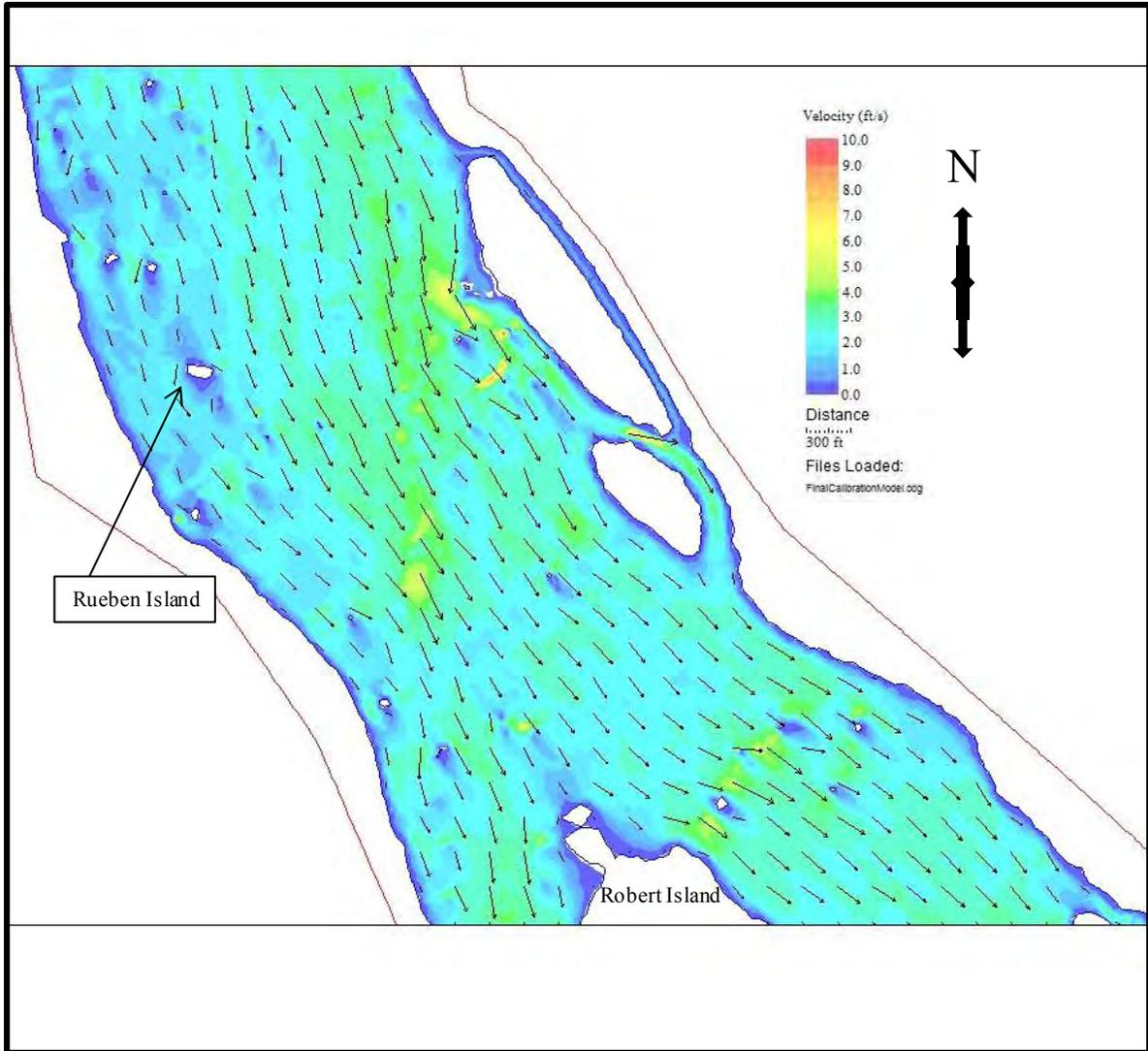
**FIGURE 4.2-10 WATER VELOCITY IN THE SUSQUEHANNA RIVER IN THE VICINITY OF SPENCER ISLAND AND ROBERT ISLAND AS DETERMINED BY RIVER 2D MODEL FOR 40,000 CFS DISCHARGE FROM CONOWINGO DAM.**
