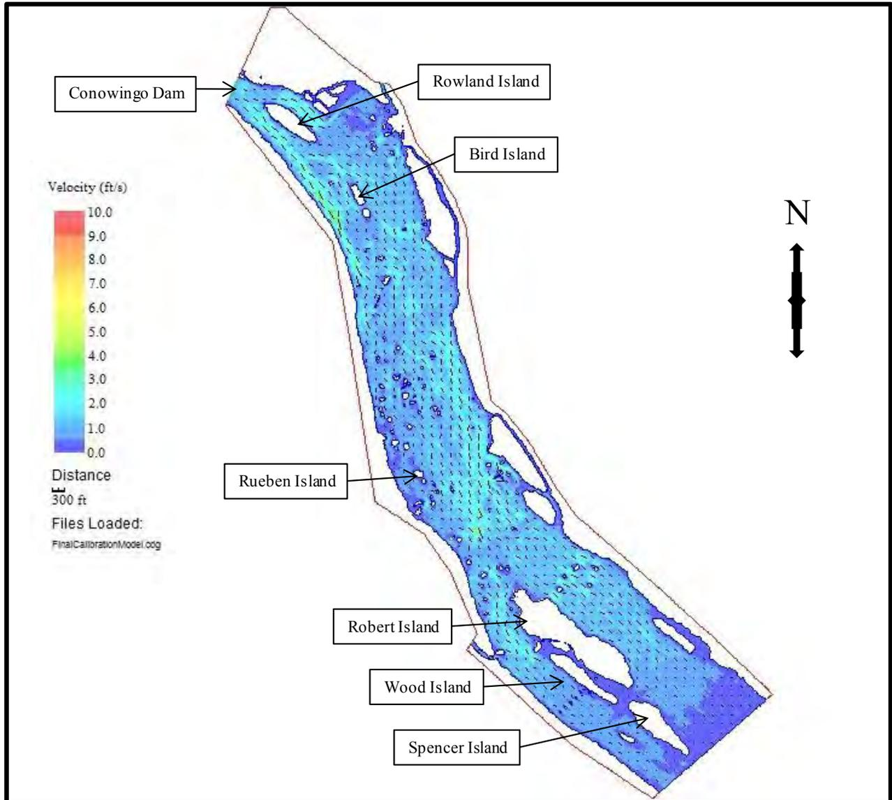
**FIGURE 4.2-2: WATER VELOCITY IN THE SUSQUEHANNA RIVER IN THE VICINITY OF ROWLAND ISLAND AND BIRD ISLAND AS DETERMINED BY RIVER 2D MODEL FOR 10,000 CFS DISCHARGE FROM CONOWINGO DAM.**
