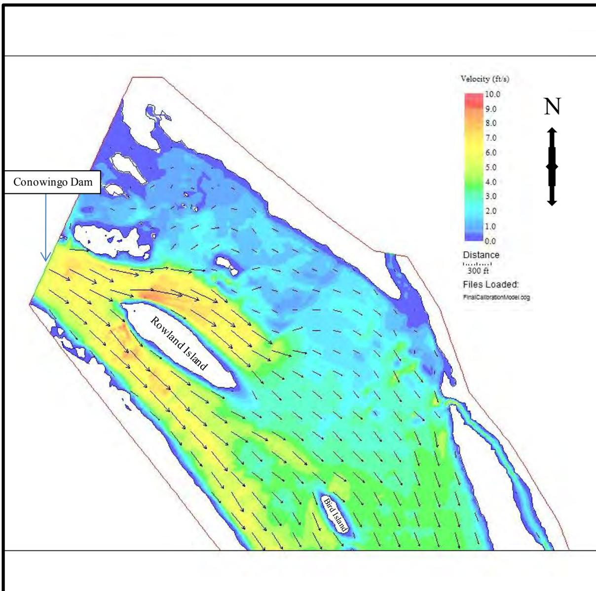
**FIGURE 4.2-13: WATER VELOCITY IN THE SUSQUEHANNA RIVER IN THE VICINITY OF BIRD ISLAND AND REUBEN ISLAND AS DETERMINED BY RIVER 2D MODEL FOR 86,000 CFS DISCHARGE FROM CONOWINGO DAM.**
