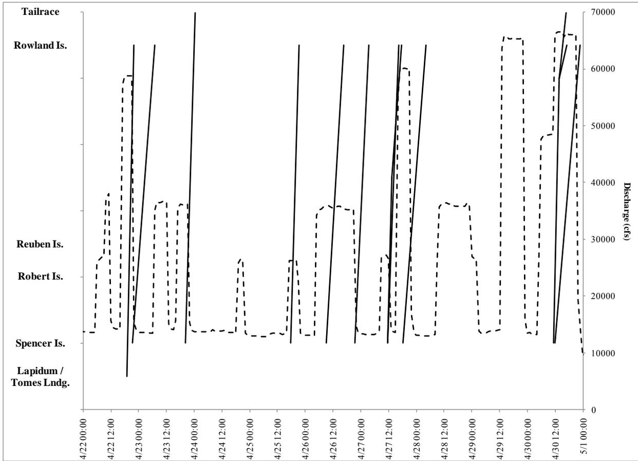
Discharge is represented by the dashed line and is USGS data from gage #01578310. Fifteen separate forays are illustrated.
