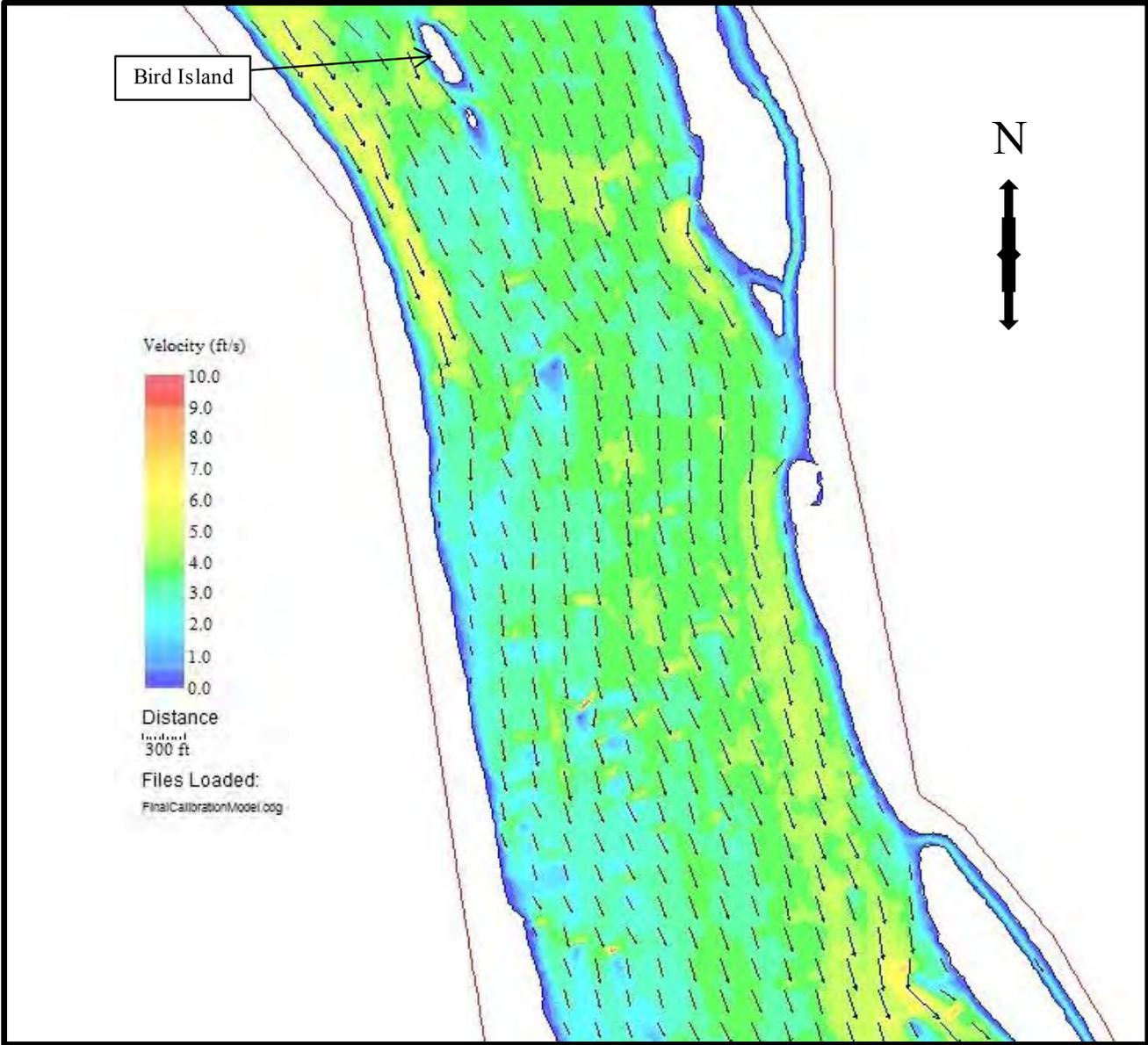
**FIGURE 4.2-14: WATER VELOCITY IN THE SUSQUEHANNA RIVER IN THE VICINITY OF REUBEN ISLAND AND ROBERT ISLAND AS DETERMINED BY RIVER 2D MODEL FOR 86,000 CFS DISCHARGE FROM CONOWINGO DAM.**
