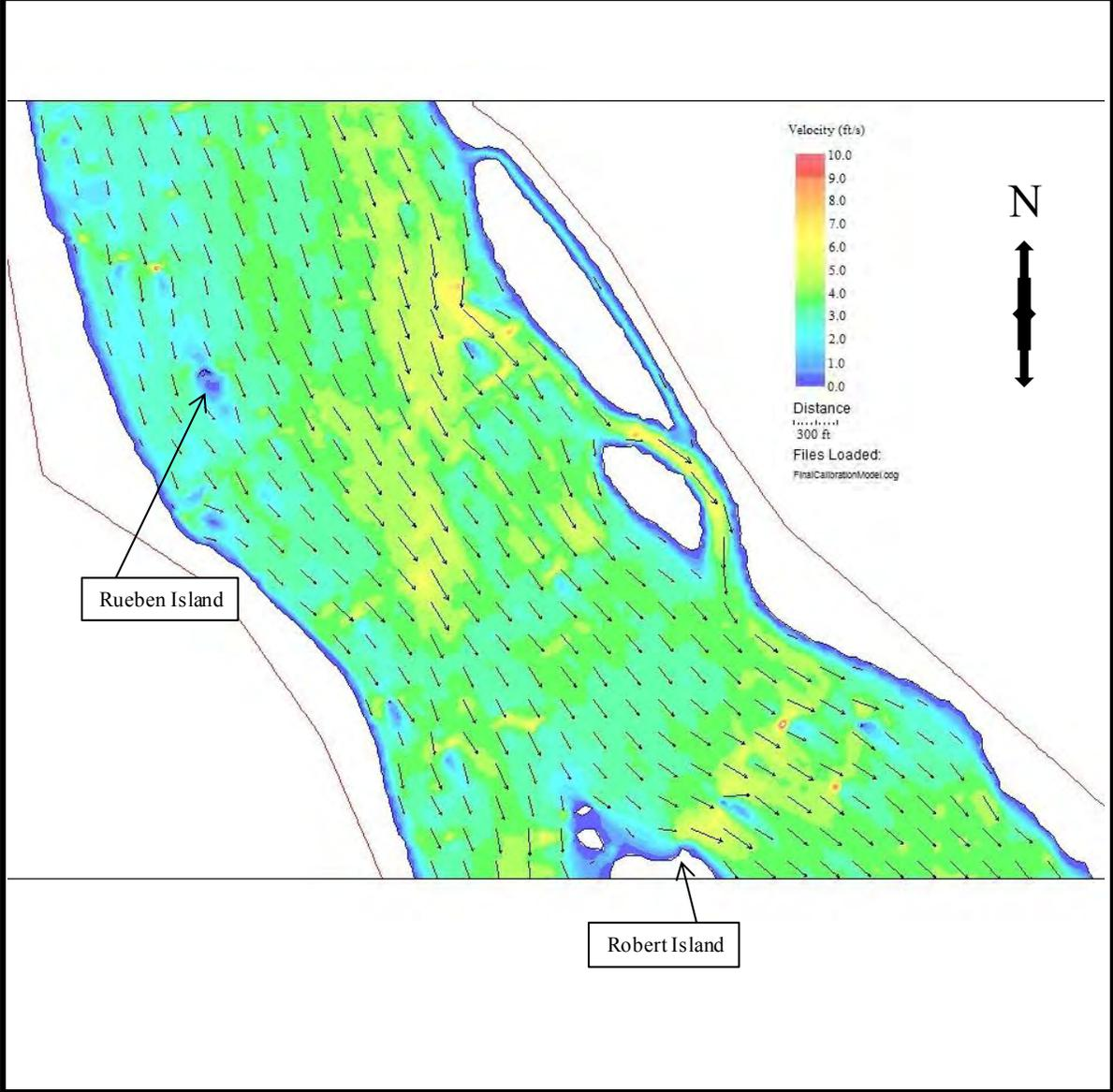
**FIGURE 4.2-15 WATER VELOCITY IN THE SUSQUEHANNA RIVER IN THE VICINITY OF SPENCER ISLAND AND ROBERT ISLAND AS DETERMINED BY RIVER 2D MODEL FOR 86,000 CFS DISCHARGE FROM CONOWINGO DAM.**
