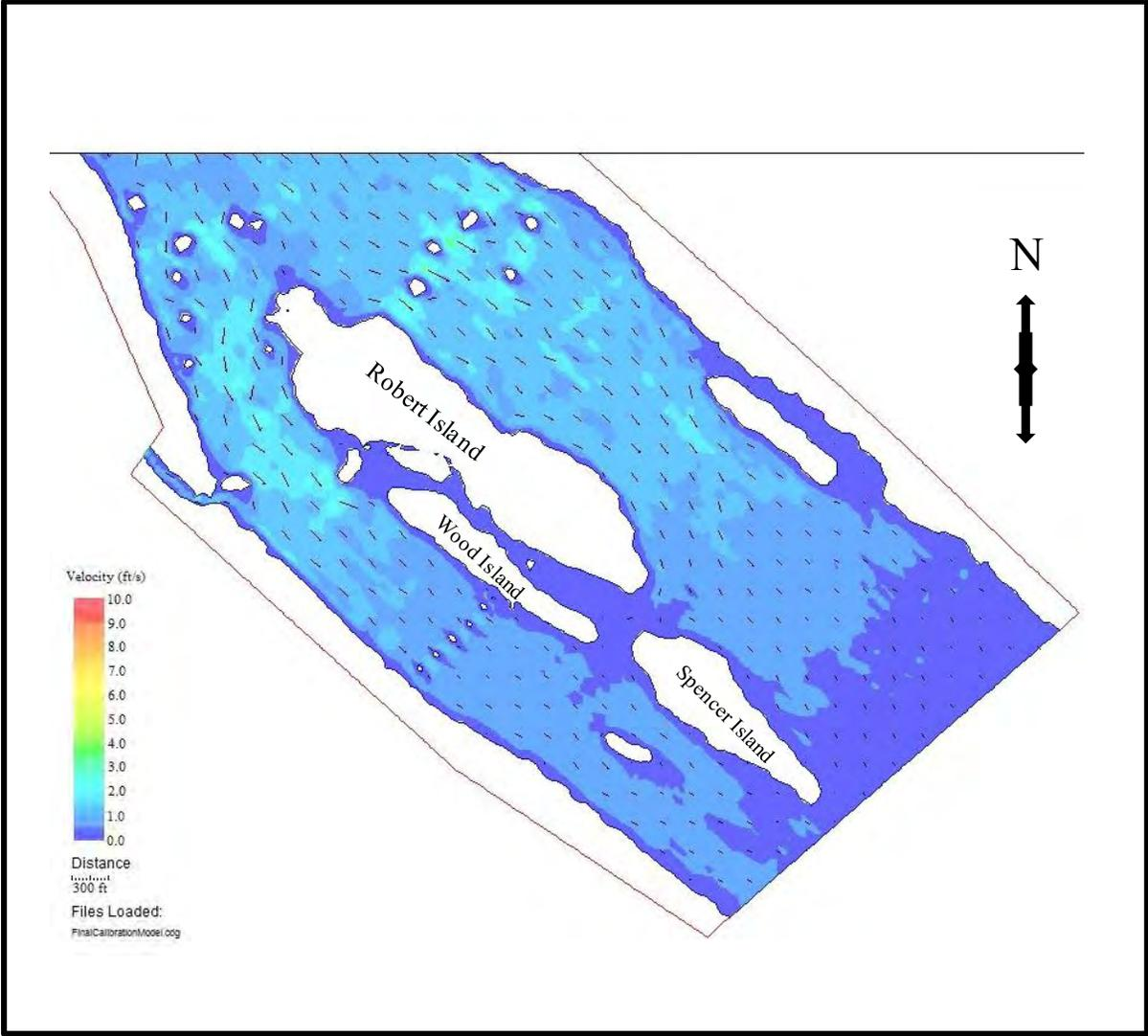
**FIGURE 4.2-6: WATER VELOCITY IN THE SUSQUEHANNA RIVER BETWEEN CONOWINGO DAM AND SPENCER ISLAND AS DETERMINED BY RIVER 2D MODEL FOR 40,000 CFS DISCHARGE FROM CONOWINGO DAM.**
