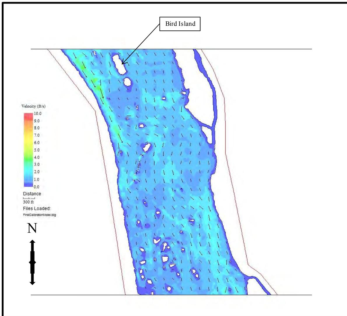
**FIGURE 4.2-4: WATER VELOCITY IN THE SUSQUEHANNA RIVER IN THE VICINITY OF REUBEN ISLAND AND ROBERT ISLAND AS DETERMINED BY RIVER 2D MODEL FOR 10,000 CFS DISCHARGE FROM CONOWINGO DAM.**
