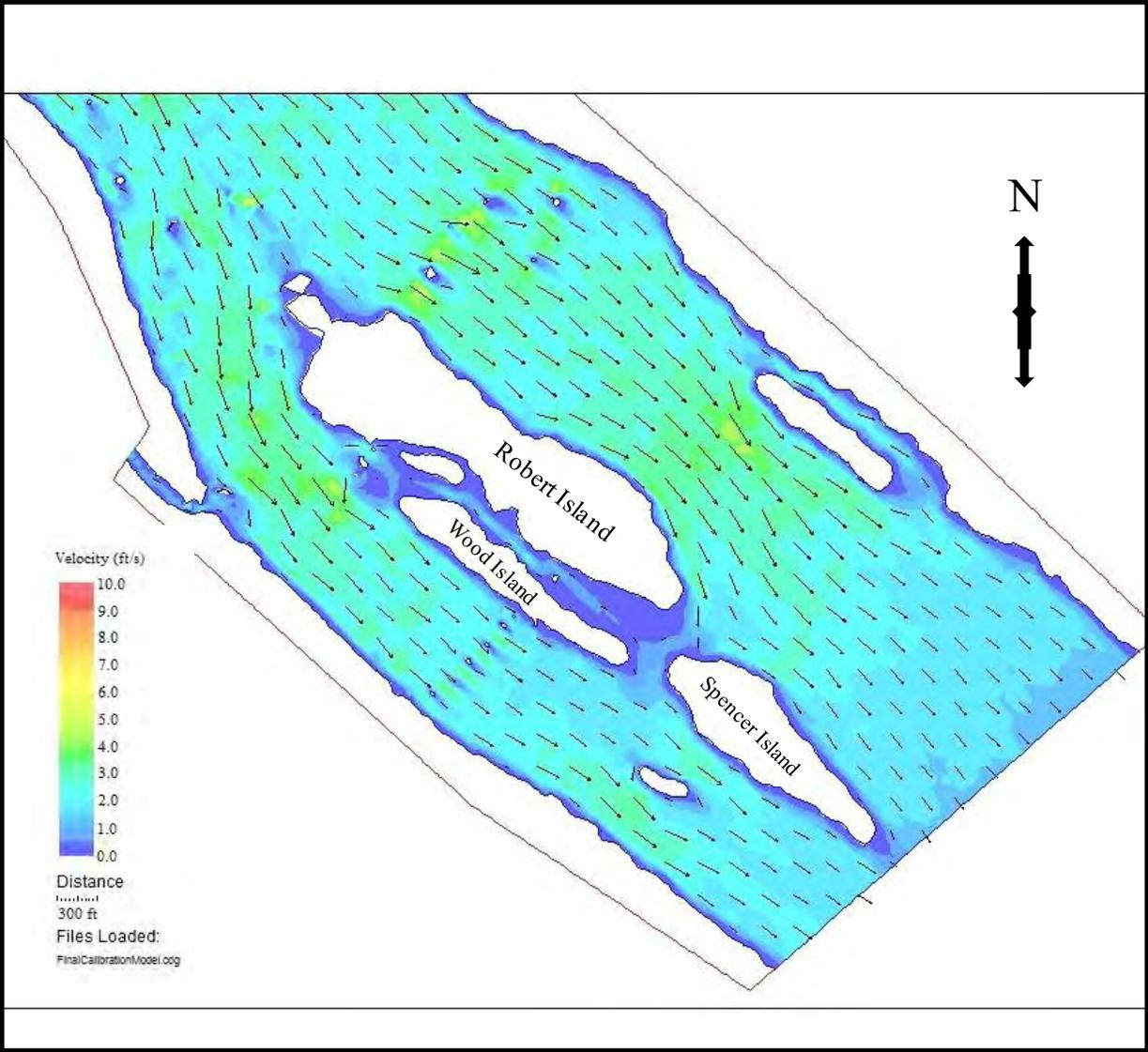
**FIGURE 4.2-11: WATER VELOCITY IN THE SUSQUEHANNA RIVER BETWEEN CONOWINGO DAM AND SPENCER ISLAND AS DETERMINED BY RIVER 2D MODEL FOR 86,000 CFS DISCHARGE FROM CONOWINGO DAM.**
