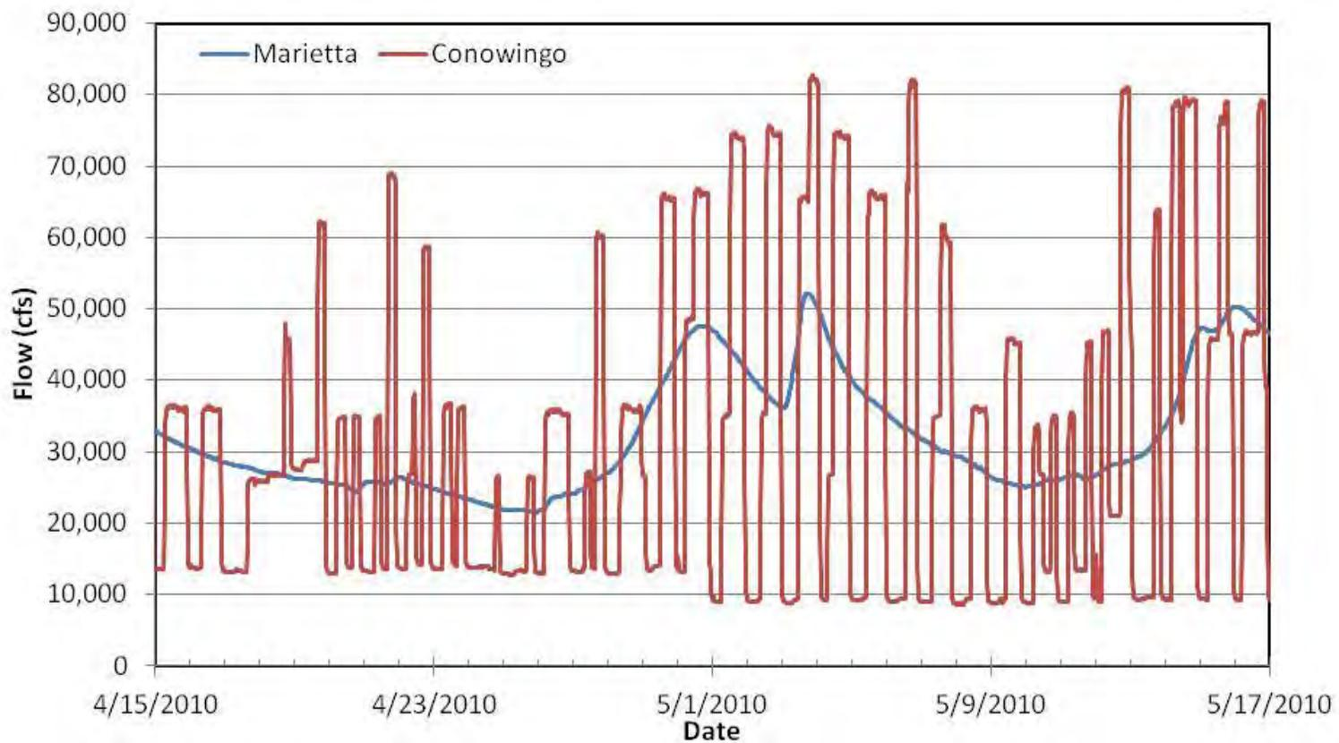
**FIGURE 3.1-3: TIME SERIES PLOT COMPARING MARIETTA AND CONOWINGO USGS GAGE FLOWS, MAY 15 TO JUNE 16, 2010.**
