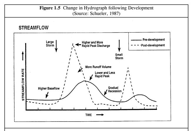
The impervious surfaces and conveyance systems of developed sites result in an earlier and higher peak discharge rate.
