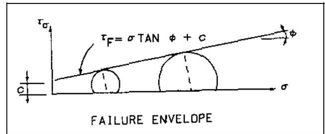
Figure 4-3. Failure envelope
