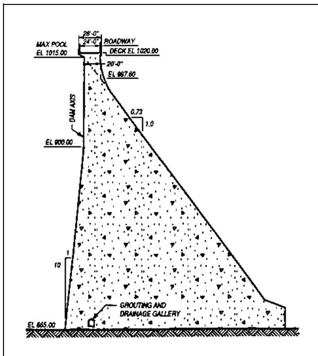
Figure 2-2. Nonoverflow section
