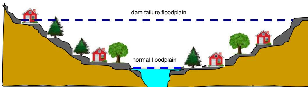
shown on the figure above. Maps of the danger reach, sometimes referred to as "inundation maps," are prepared by an engineer based on hydrologic and hydraulic analyses and topography of the affected
