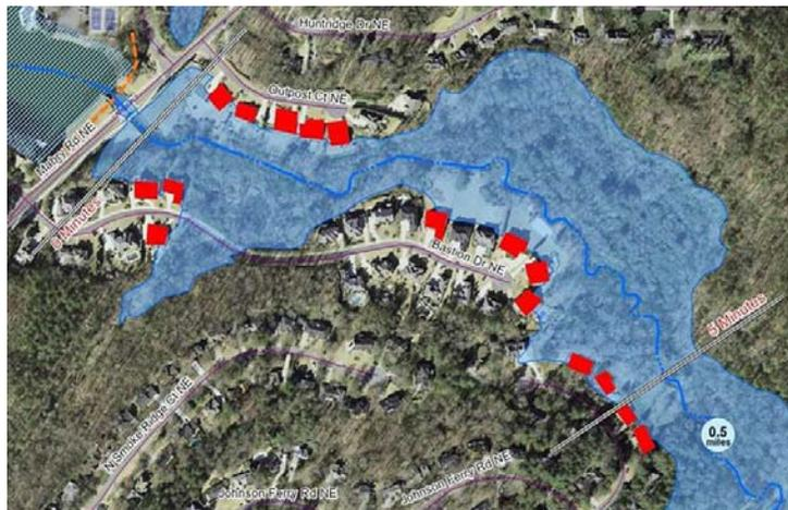
The figure above is an example of a danger reach delineation. It shows the dam in the upper left hand corner of the image, and the area expected to be inundated should the dam fail. Homes which would be flooded are shown in red.
