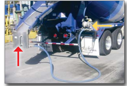
Figure 8. Chute washout bucket and pump
