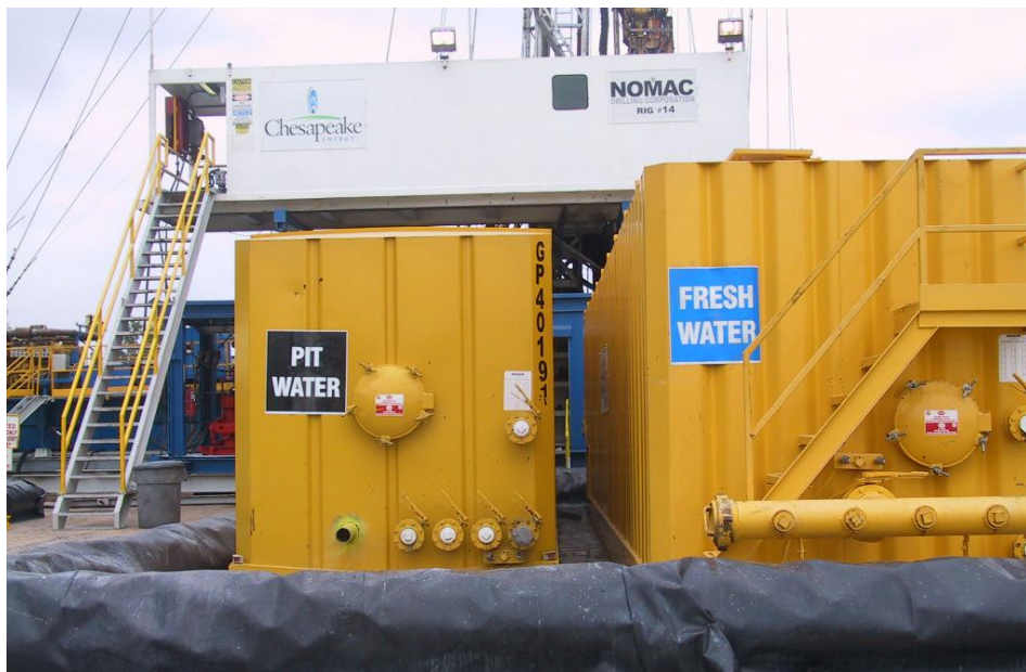
A well managed drilling operation carefully contains the pit or frac water for reuse or treatment when it can no longer be used. Many millions of gallons of freshwater are used to drill each well.
