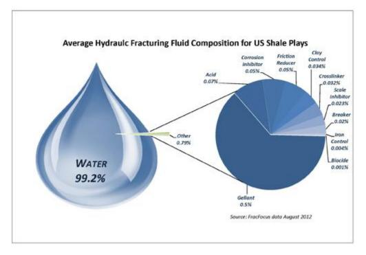
Figure 3. Average Hydraulic Fracturing Fluid Composition Source: ALL Consulting from FracFocus website, <u>http://fracfocus.org/water-protection/drilling-usage</u>
