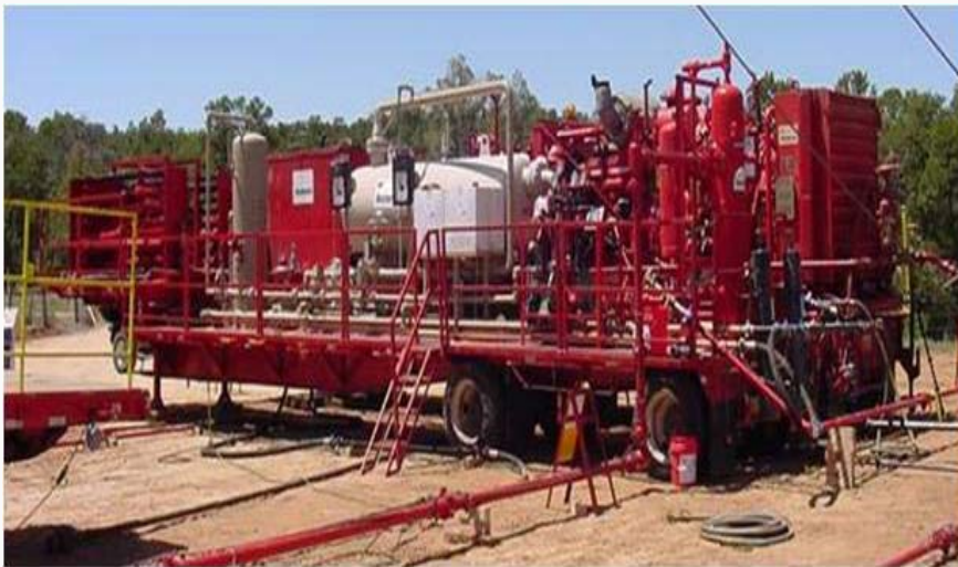
Green Completion Equipment (source: Weatherford)
