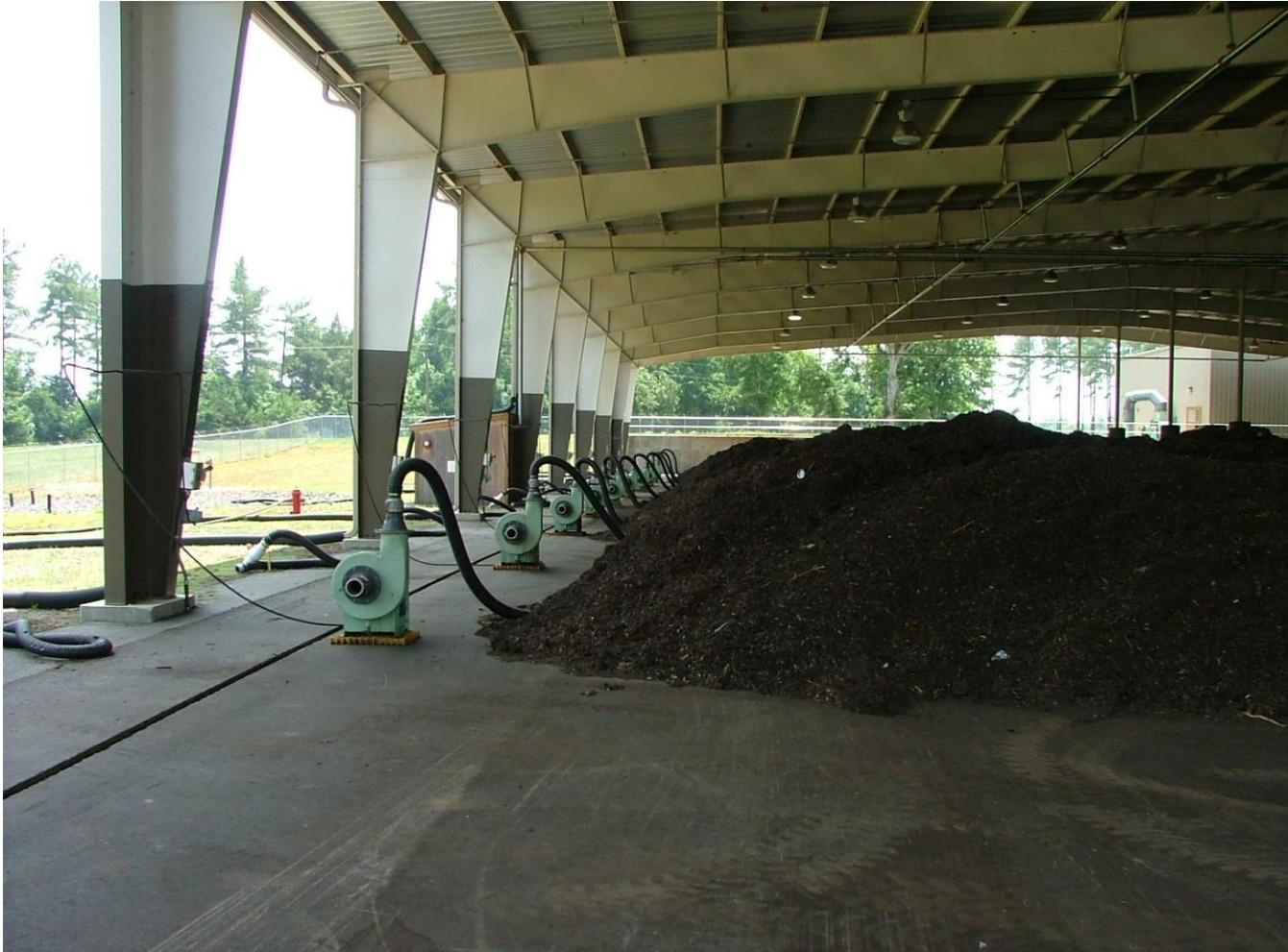
Sewage sludge and woodchips at treatment plant
