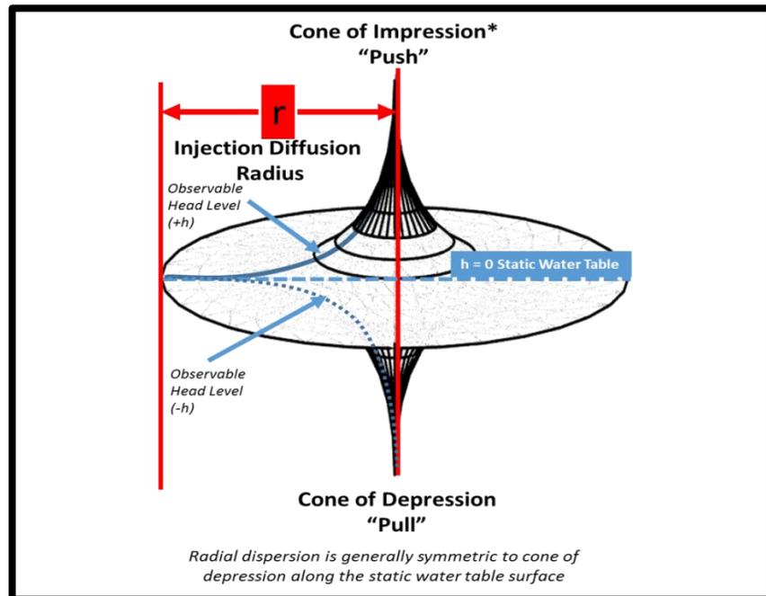
Under the generalized radial dispersion model, if  $Q$  and  $K$  are constant, at a monitoring well within the Injection Diffusion Radius, one can record and document the following to assure hydraulic recovery:
