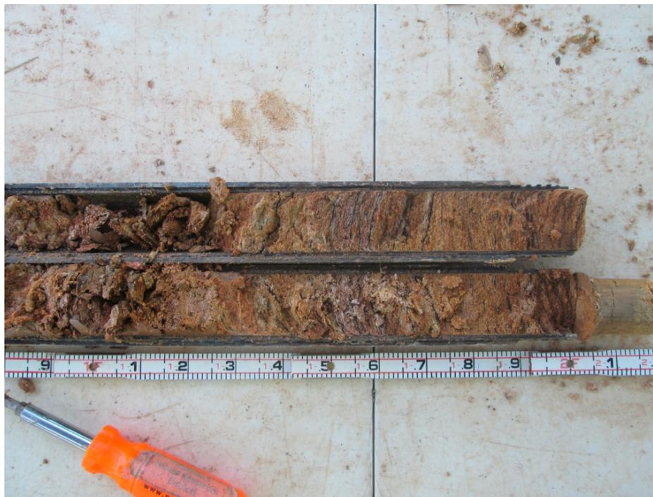
**PHOTO 3: Structured saprolite – MW-6D - July 10, 2015**
