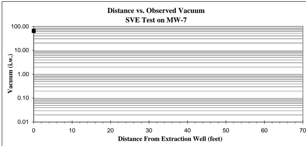
NOTE: No significant vacuum was observed. Therefore the ROI is estimated at "Less than 24 feet".
