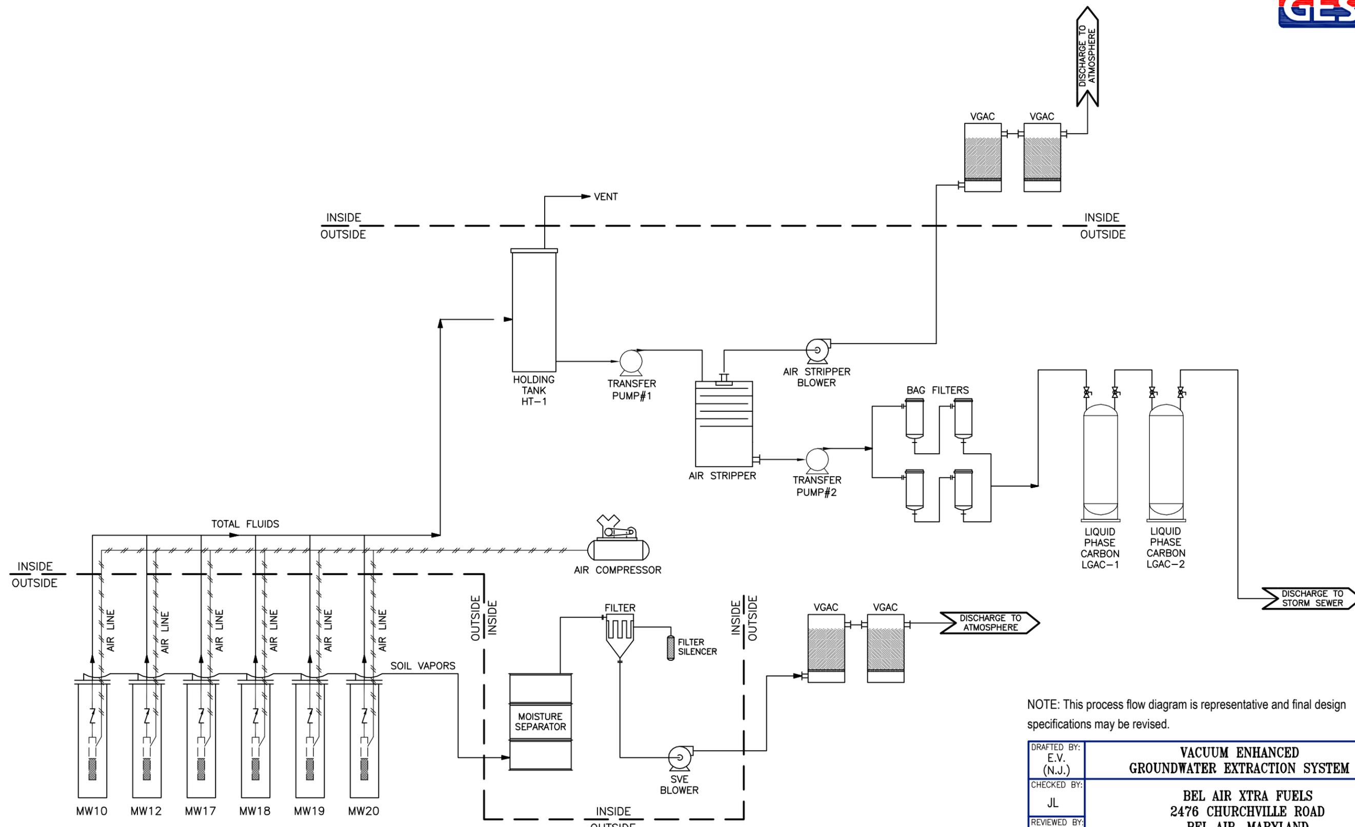
NOTE: This process flow diagram is representative and final design specifications may be revised.
