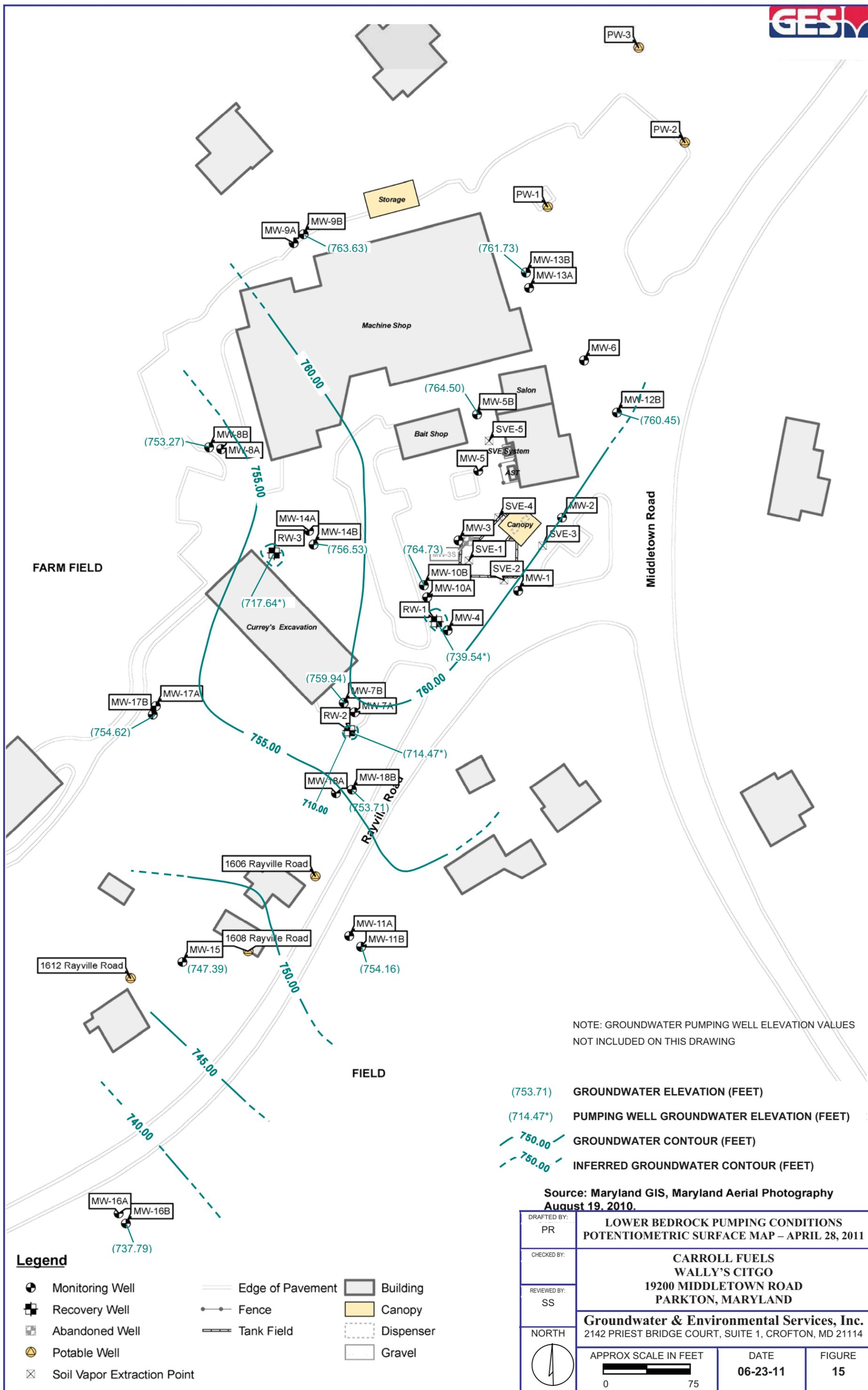
NOTE: GROUNDWATER PUMPING WELL ELEVATION VALUES NOT INCLUDED ON THIS DRAWING
