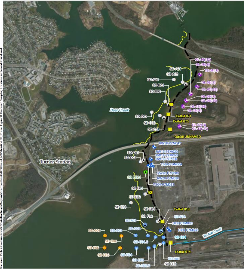
Figure 11 Proposed Sampling Locations for the Second Round of the Offshore Investigation Phase I Northwest Shoreline Baltimore, Maryland Legend Phase I Northwest Shoreline Perennial Creek/Stream Boundary between Sand and Fine Grained Sediment Round 1 Sediment Sampling Location Proposed Surface Sediment Sampling Location Proposed Sediment Coring Location Proposed Sediment Coring Contingency Location Proposed Pore Water Sampling Location Greys Landfill Well Groundwater Well Sampled in June 2014 Approximate Location of Active Stormwater Outfall Approximate Location of Inactive Stormwater Outfall Map Date: January 2015 Image Source: ESRI 2011 Projection: NAD 1983 StatePlane Maryland FIPS 1900 (US Feet) 0 300 600 1,200 Feet 1 inch = 1,200 feet
