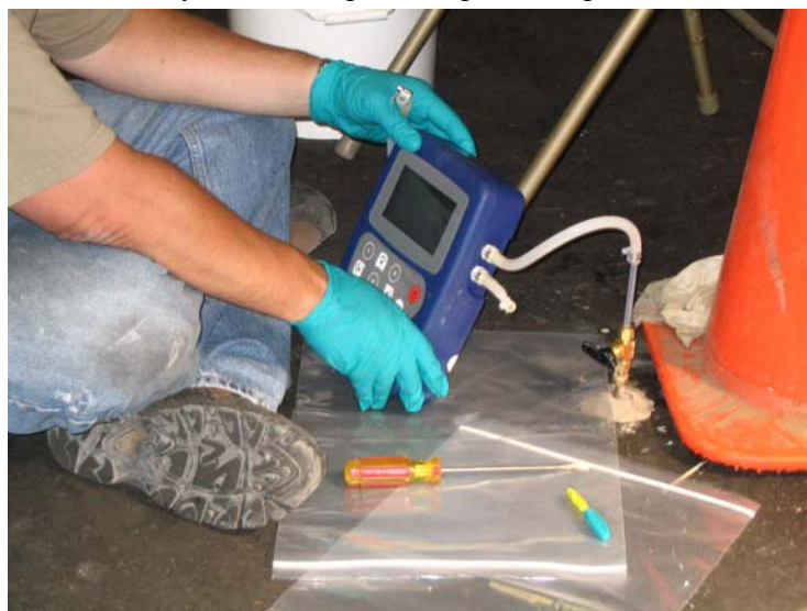
Figure 2—Sub-slab Gas Samples Collected
