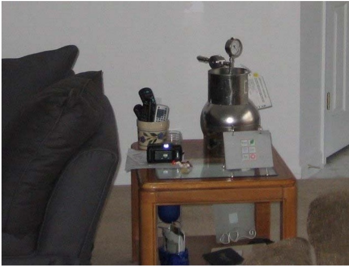
Figure 3—Indoor Air Samples Collected Using a Summa Canister
